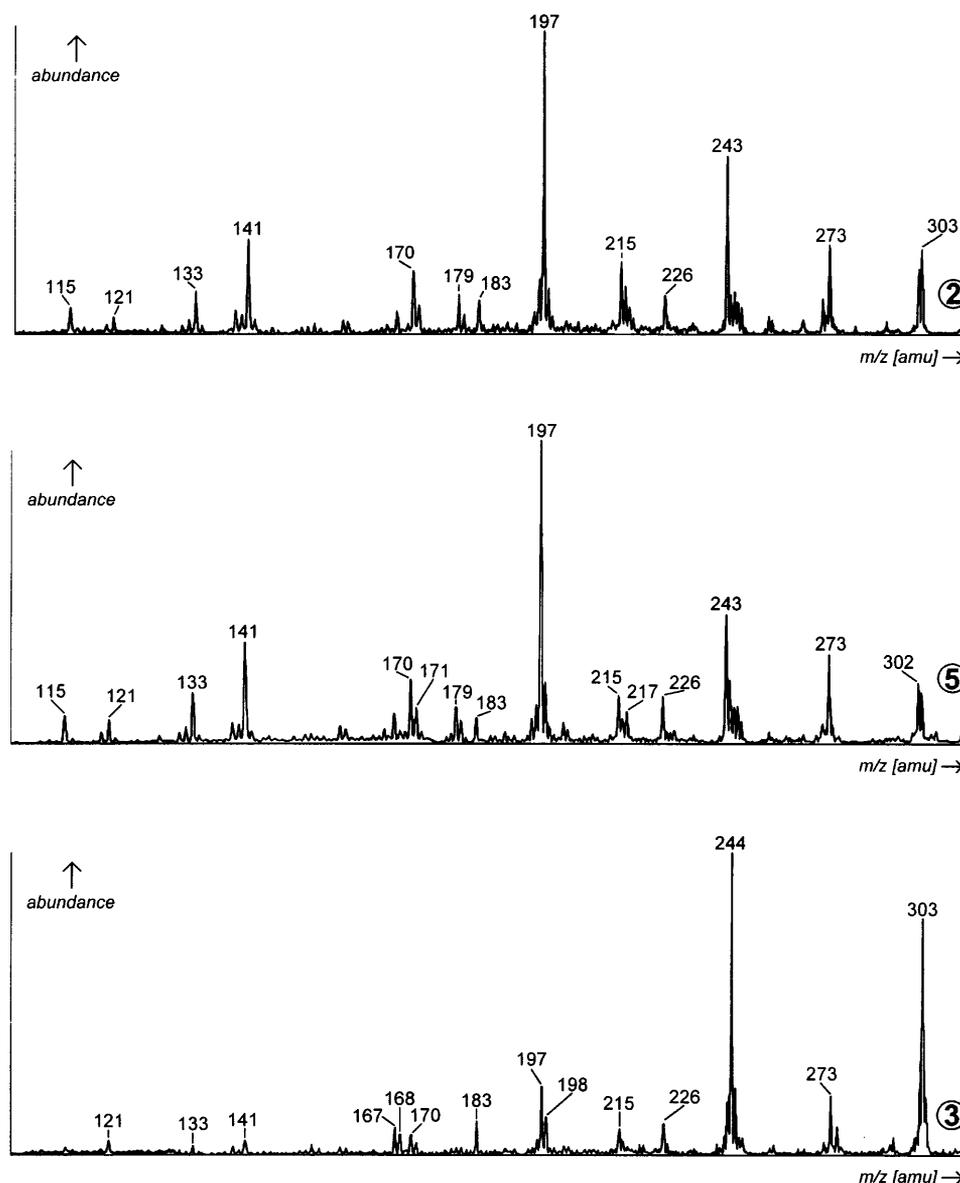
Figure 1. CAD mass spectra of the ions at  $m/z$  321 originating from **2** (top), **5** (middle) and **3** (bottom).
