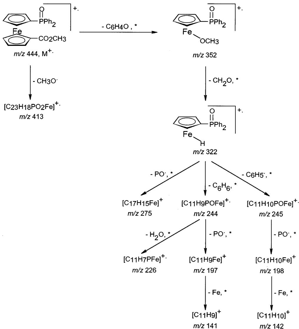
Scheme 6. Fragmentation scheme for carboxy phosphine oxide methyl ester **6**.
