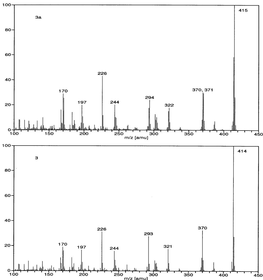
**Figure 2.** EI (80 eV) mass spectra of carboxyphosphine **3** and its deuterated analogue **3a**. The deuteration degree of only ~60% was reached due to a fast H/D exchange of active hydrogen atoms.
