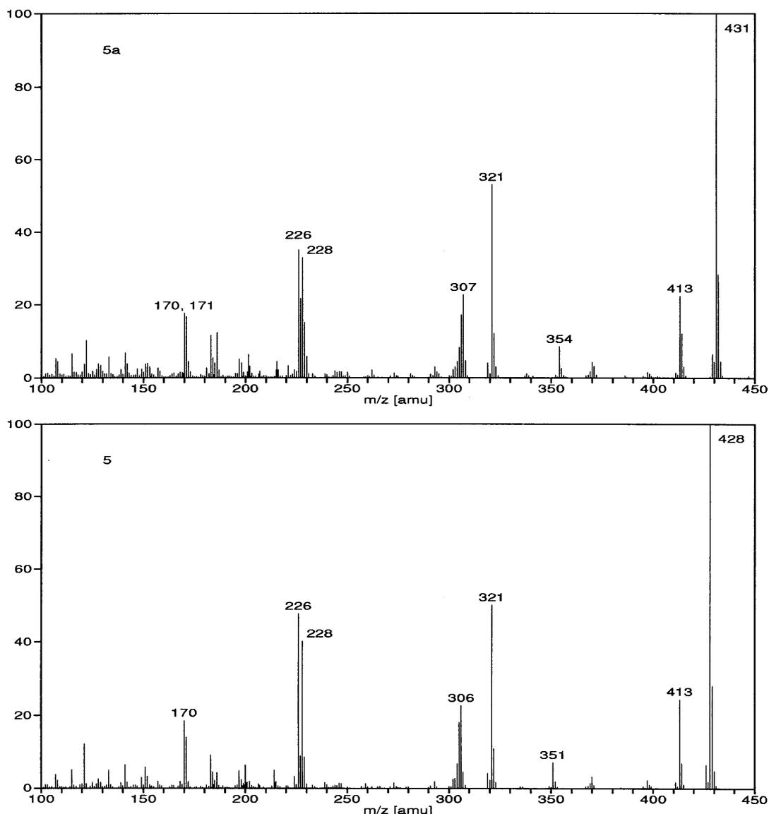
Figure 3. EI (80 eV) mass spectra of carboxyphosphine methyl ester **5** (bottom) and its  $d_3$ -isotopomer **5a** (top).
